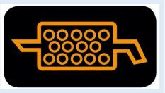
successfully, the vehicle is required to run for a prolonged period or risk the DPF becoming clogged and ultimately fail. Other reasons for DPF failure include ineffective heater plugs or underlying engine problems.
